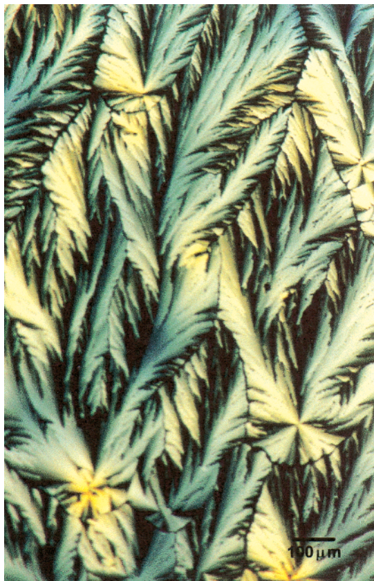
Figure 1. Texture of a sample of 4 between crossed polarizers at 300 °C. Magnification, 200 \times .
